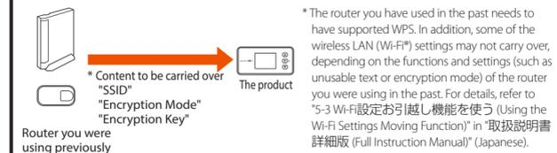
\* The router you have used in the past needs to have supported WPS. In addition, some of the wireless LAN (Wi-Fi®) settings may not carry over, depending on the functions and settings (such as unusable text or encryption mode) of the router you were using in the past. For details, refer to "5-3 Wi-Fi設定お引越し機能を使う (Using the Wi-Fi Settings Moving Function)" in "取扱説明書 詳細版 (Full Instruction Manual)" (Japanese).
